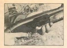
Speed-load by rolling the shell into the empty chamber from underneath receiver, then sliding forward to close the action.
